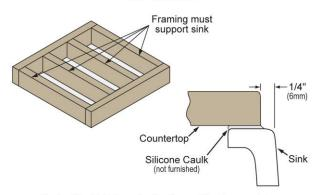
Designed to affix to the underside of any solid surface countertop.
